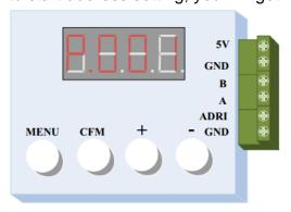
**Step 3**: 'P:001' means the original/start DMX address is '1'. Please press key '+' to adjust the original address at your request.
